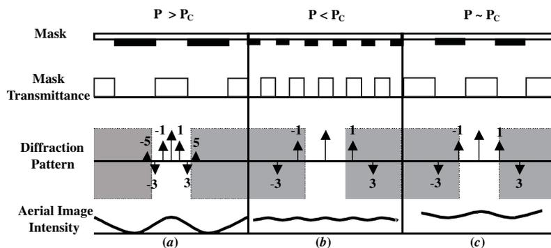
**Figure 2.** Illustration showing behavior of diffracted light assuming the critical pitch  $P_C$  is the smallest pitch where the numerical aperture accepts one of the first diffraction orders. Diffraction orders in the shaded region denote the orders not accepted by the numerical aperture of the objective lens in the lithography system.
