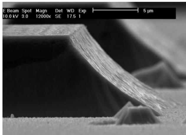
**Figure 14.** SEM image of an etched silicon structure resulting from a gray-scale nested mask and RIE etching using a pitch of  $3.5 \mu\text{m}$  and one row per pixel size.
