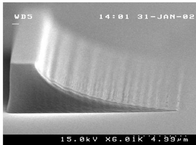
**Figure 8.** SEM image showing developed AZ 4620 photoresist using a  $3.5\ \mu\text{m}$  pitch and one row per pixel size.
