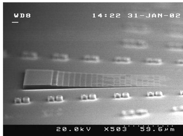
**Figure 6.** An SEM image of AZ 4620 developed photoresist consisting of 22 height levels using a  $3.5 \mu\text{m}$  pitch on the mask and ten rows per pixel size.
