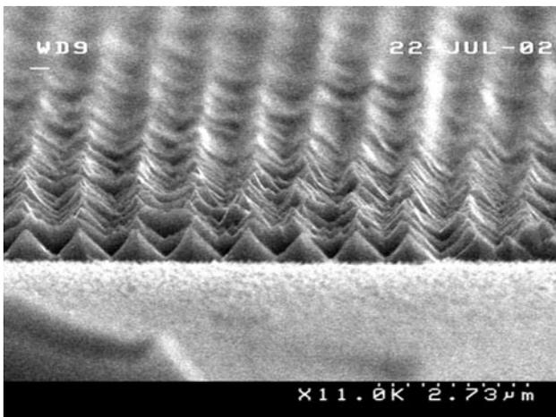
**Figure 11.** SEM image of the lowest gray level corresponding to the silicon structure in figure 8. The spaces between the spikes seem to reach the surface of the silicon that was not masked by photoresist.
