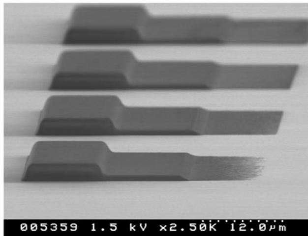
**Figure 4.** Three gray levels patterned in AZ 4620 photoresist resulting from a similar mask pattern in figure 3.
