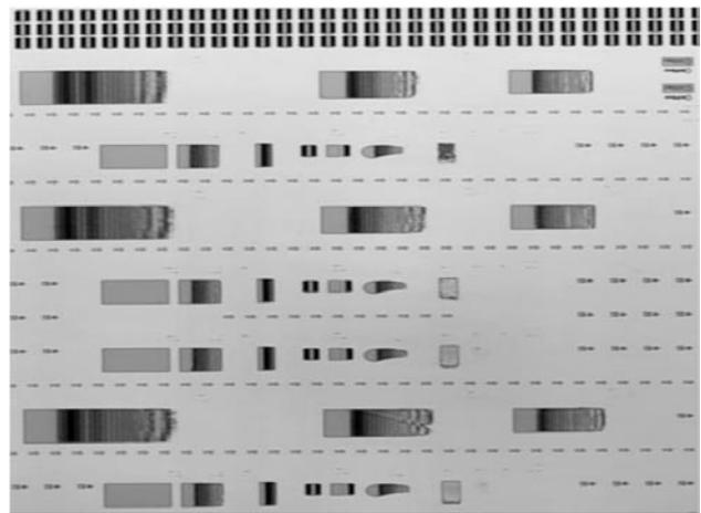
**Figure 5.** An optical micrograph showing a top down view of the gray-scale mask layout developed in AZ 4620 photoresist.
