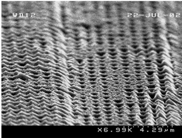
**Figure 10.** SEM image of the thicker gray levels etched in the silicon corresponding to the structure shown in figure 9. This SEM shows the surface roughness, which comes from the holes in the photoresist layer due to the intensity oscillations.
