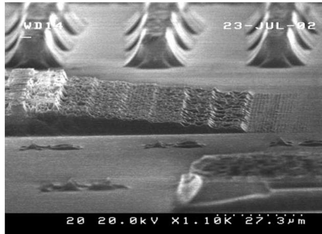
**Figure 12.** SEM image of a silicon etched structure about  $11 \mu\text{m}$  tall resulting from a higher selectivity and a lower chamber pressure etch. A total of ten gray levels were achieved using this etch.
