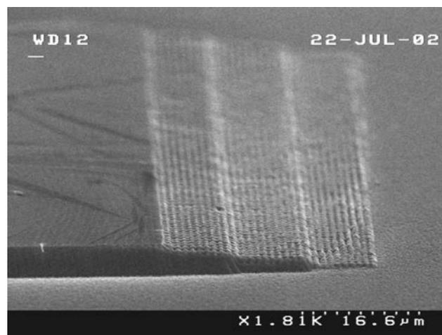
**Figure 9.** SEM image of an etched silicon structure  $9\ \mu\text{m}$  tall resulting from a gray-scale nested mask and RIE etching using a pitch of  $5.0\ \mu\text{m}$  and ten rows per pixel size.
