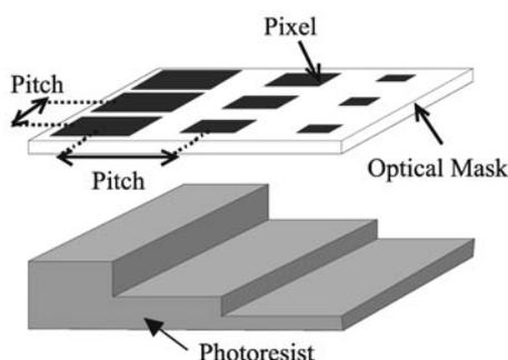
**Figure 3.** Example of a three-level gray-scale mask pattern and the resulting photoresist structure.
