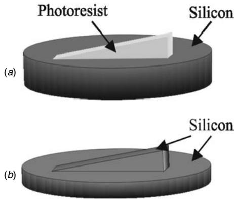
**Figure 1.** An illustration showing the two primary steps for the fabrication of arbitrary 3D silicon structures using gray-scale lithography to form a nested mask. In (a), exposed and developed photoresist from gray-scale lithography for use as a masking layer is shown. In (b), the final RIE etched structure in silicon is shown using the masking layer from (a).
