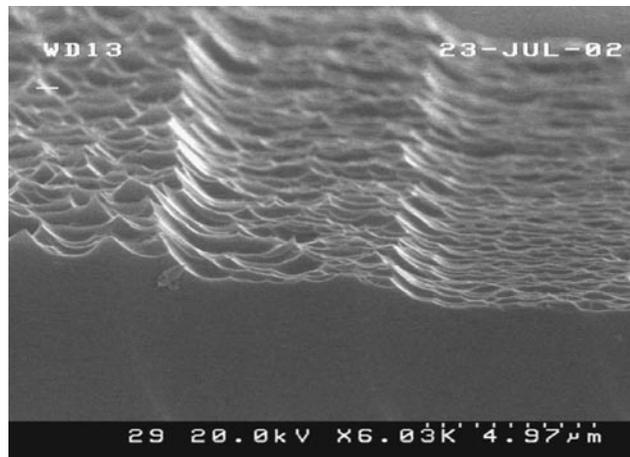
**Figure 13.** SEM image showing a close-up view of the upper levels that are shown in figure 12. From the etch process used, the roughness has been decreased and there are no periodic spikes.
