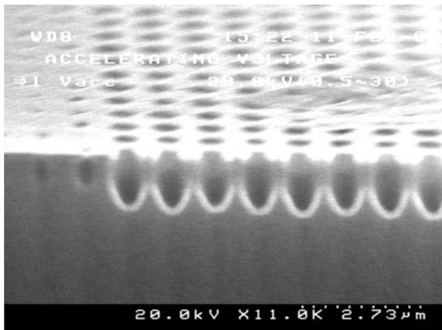
**Figure 7.** SEM image showing holes in an upper gray level developed in AZ 9245 photoresist due to the partial recreation of the features.
