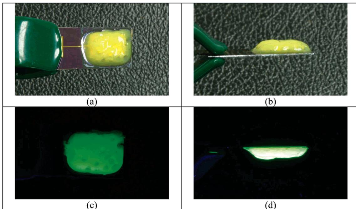
**Figure 1.** Chitosan hydrogel deposited on a patterned gold cathode: (a) top and (b) side views; (c) top and (d) side views using a UV light source. Deposition was carried out using 1.5% w/w fluorescently labeled chitosan of bulk pH = 5.5 for 20 min at a current density of 50 A/m<sup>2</sup>. The thickness (i.e. height) of the deposit was estimated to be 5 mm. The “pores” created by the evolved gas bubbles are evident in these photos.
